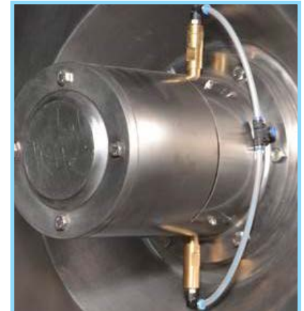
Air Purged Sanitary Sealing
